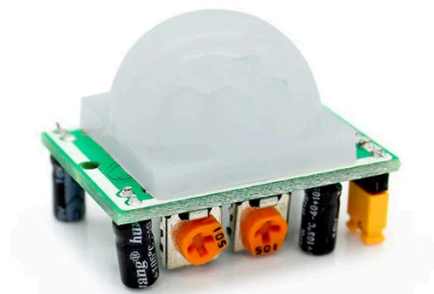
Figure 02: PIR HC-SR501 motion sensor
